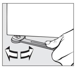
Turn the 4 screw feet to adjust the dryer to the correct height and level.
